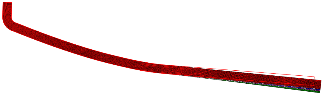
Figure 6.17: Blank configurations before springback with different mass scaling factors
