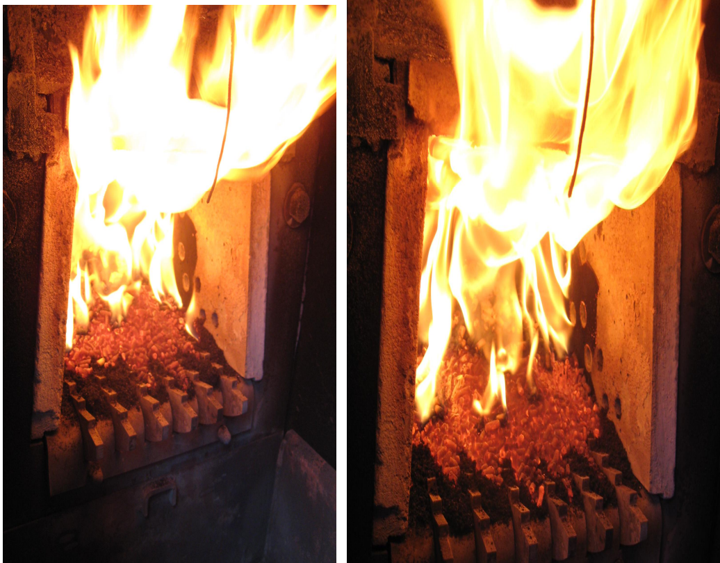
Figure 5.3. On the left hand side, fuel bed in the combustion chamber after the 18 revolutions. On the right hand side, fuel bed in the combustion chamber after the 9 revolutions.
