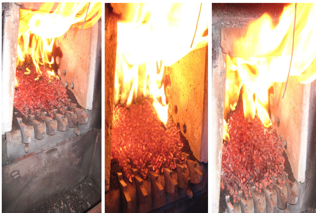
Figure 5.4. On the left fuel bed after the 6 revolutions step; in the middle, fuel bed after the 4 revolutions step; on the right fuel bed after the 3 revolutions step.
