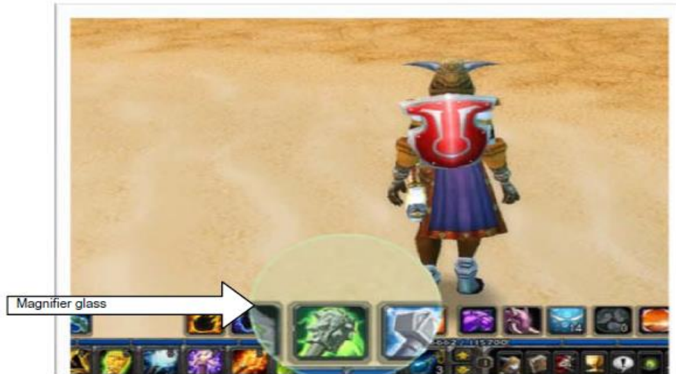
Figure 8 - Magnifier class to help selecting from the icons (Source: Istance et al. 2009)
