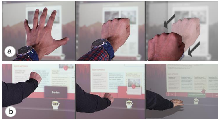
Figure 15. Interaction techniques to retrieve content from public display: (a) Grab & Pull: ‘Grab’ an element on the screen and ‘Pull’ the element from the screen, (b) Grab & Drop: ‘Grab’ an element on the screen, drag it and drop it over the specified drop area.
