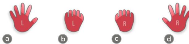
Figure 18: Different states of hand cursor : (a) Left hand open (pointing, release). (b) Left hand closed (grabbing). (c) Right hand closed (grabbing). (d) Right hand open (pointing, release).
