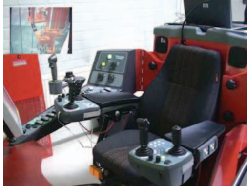
Fig. 1. Drill rig simulator with a picture of the user's view attached to the top left
