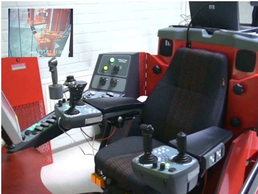
Figure 7. The evaluation environment of the DrillSimulator case (II): The user sits on the seat and sees the view attached to the top-left corner on a screen in front of him (Keskinen, Turunen, Raisamo, Evereinov, & Haverinen, 2012, Figure 1, © Springer Berlin Heidelberg 2012).
