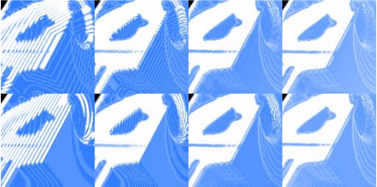
Figure 21 Rendering quality difference between ray casting (upper row) and slicing (bottom row) with 64 (left), 128, 256 and 512 (right) steps.
