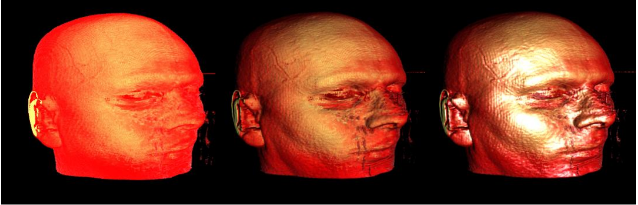
Figure 13 Illumination effect to the rendering (left image: no illumination, middle image: illumination with the diffuse term, right image: illumination with the diffuse and the specular term)
