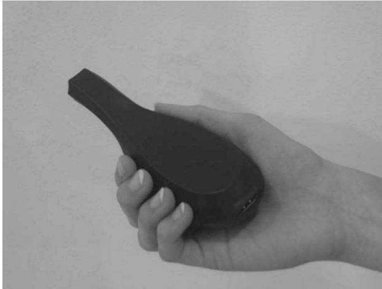
Figure 3. A picture of a prototype capable of producing vibrotactile stimulation used in the current thesis. One vibrotactile actuator is embedded inside the device and two are on the surface of both sides.
