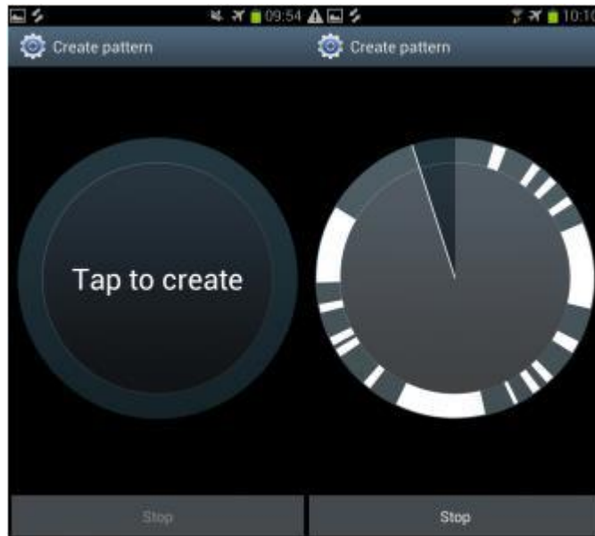
Fig 6. In Auto Haptic the user taps the circle to create unique vibration patterns.
