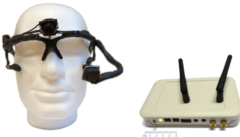
Figure 8. Face Interface prototype: On the left the wearable part and on the right the unit for the wireless functionality. Figure adapted from Publication IV.
