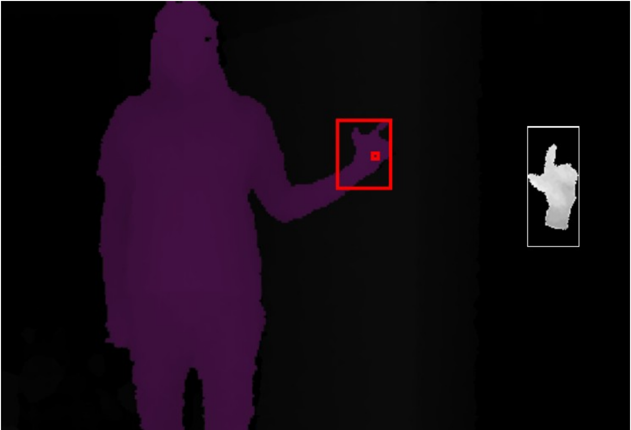
Figure 10. Left: Hand held in the L-shaped activation gesture, red dot showing the cursor position and red square signifying recognized hand gesture. Right: hand gesture data collected and reordered to upright position from 39 degree angle.
