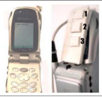
Figure 7: ChordTap prototype. The right image shows the chord keys mounted on the back of the phone. [Widgor and Balakrishnan, 2004].
