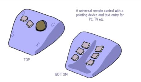
*Figure 31:* A sketch of a GKOS remote control combining a pointing device and a GKOS text entry method [GKOS-1, 2010].
