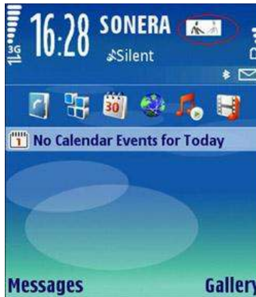
Figure 32: ACSEH-Displaying sharing session icon to indicate that sharing session is still active [Belimpasakis et al., 2008b]
