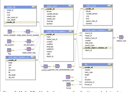
Figure 9: Media DB tables for the storage of media object and relation data.
