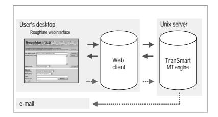
Figure 4. Basic architecture of Roughlate.
