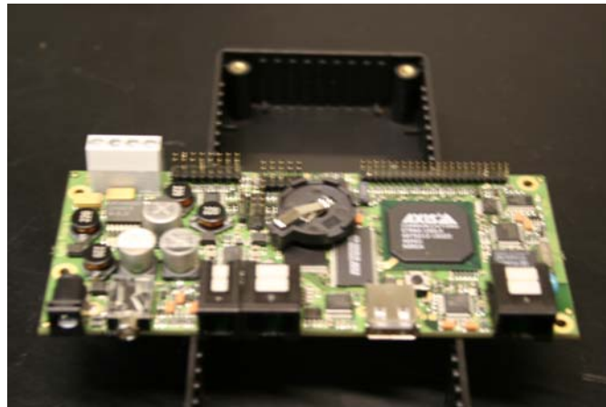
Figure 7.8. Linux server integrated on a small size circuit board.
