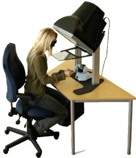
Figure 2.23. Example of haptic interaction. A user uses a Phantom device (SensAble, 2007) with a Reachin display (Reachin, 2007) to navigate in 3D space.
