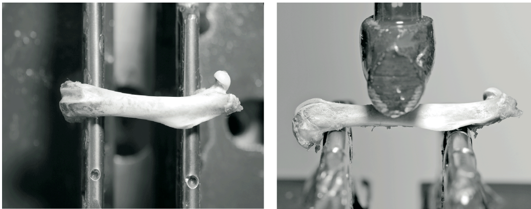
Figure 13. Three-point bending test of the femoral midshaft.
