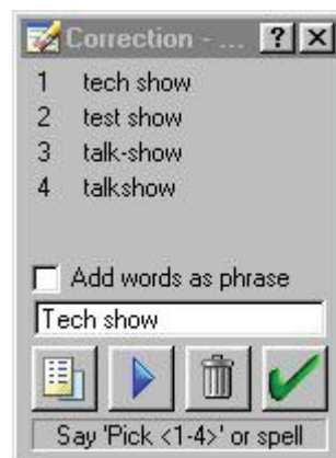
Figure 3. Error correction window from IBM ViaVoice. The window presents an N-best list after a user activates the error correction with the “Correct that” command.
