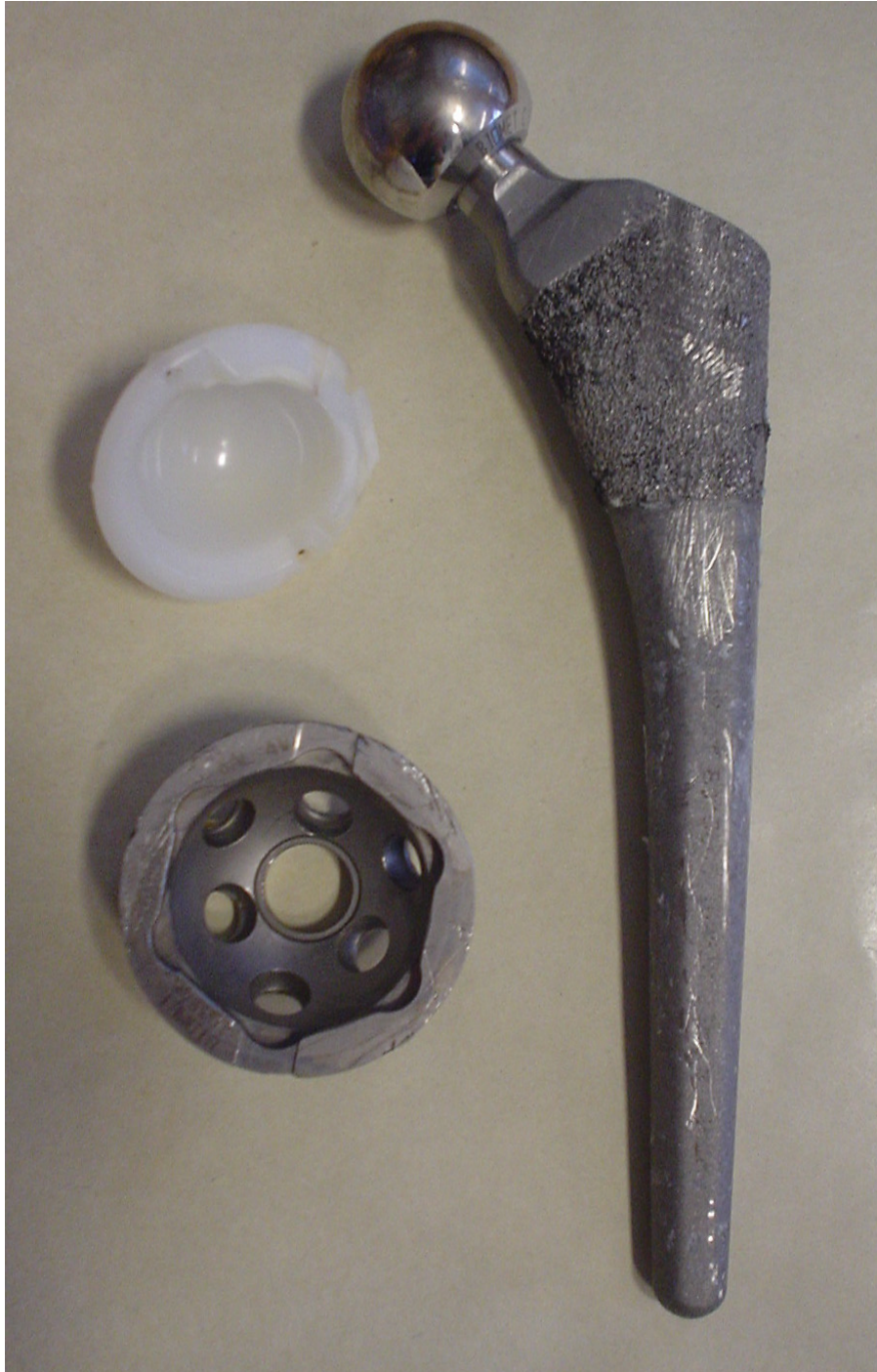
Figure 2. Retrieved Biomet Bi-Metric stem, Universal cup and Hexloc liner.
