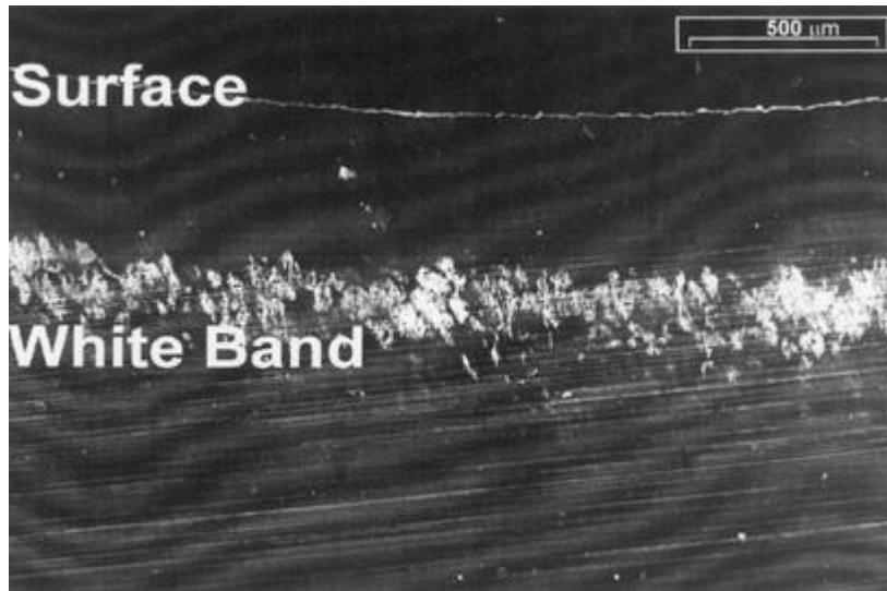
Figure 12. Subsurface white band in the optical dark field micrographs. (From Puolakka et al: Increased volumetric wear of polyethylene liners with more than 3 years of shelf-life time. Int Orthop. 2003;27:153-9).
