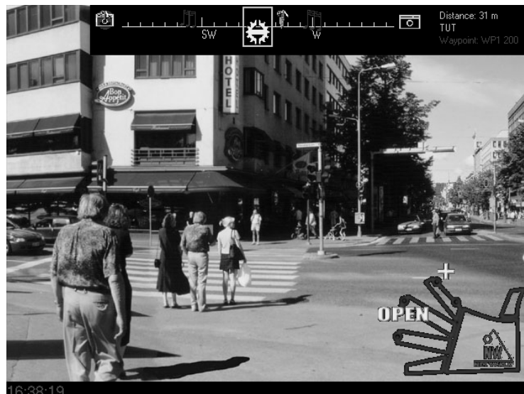
Figure 17. The Context Compass is displayed at the top of the screen. This is a synthesized image as it would appear through the head-worn display.
