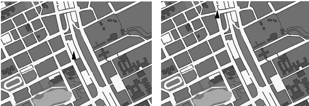
Figure 1. The behavior of the YAH symbol in two cases when the user moves. In the lefthand picture, the YAH remains in the middle of the screen and the map moves, whereas in the righthand picture the map remains static and the YAH symbol moves.
