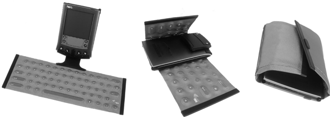
Figure 5. A folding soft keyboard for Palm Pilot hand-held computer by ElectroTextiles. Photo by courtesy of Electrotexiles Company Ltd.
