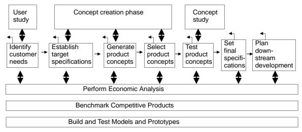
*Figure 4.6.* Needs identification, target specifications, and various conceptual phases in concept design (Ulrich and Eppinger 2000).
