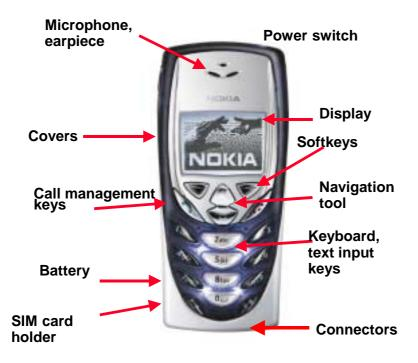
Figure 4.3. Mechanical components in a mobile phone user interface (Nokia 8310).
