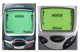
*Figure 4.4*. Nokia 7110 (left) has two softkeys and a "roller" for UI navigation. Call handling keys are green and red buttons. Nokia 3110 (right) has one softkey and up/down arrows for navigation. No special keys for call handling.
