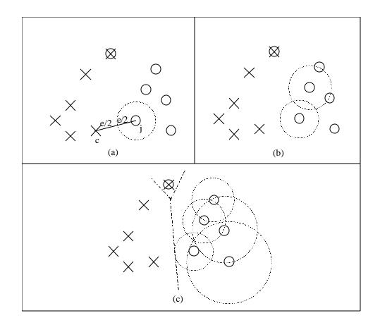
Figure 6. Example of how the hypersphere method builds a complex decision volume in 2-dimensional Euclidean space. Length of radiuses are half of distances to the nearest case that come from another class.
