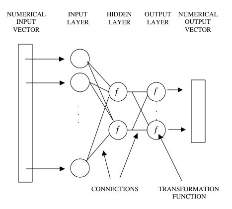
Figure 1. Feed forward multilayer perceptron neural network and its basic elements.
