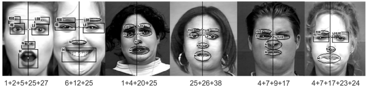
Figure 3. Examples of correctly localized facial landmarks in “face only” and “face & hair” datasets. Images are courtesy of the Cohn-Kanade AU-Coded Facial Expression database [8]. Reprinted with permission.
