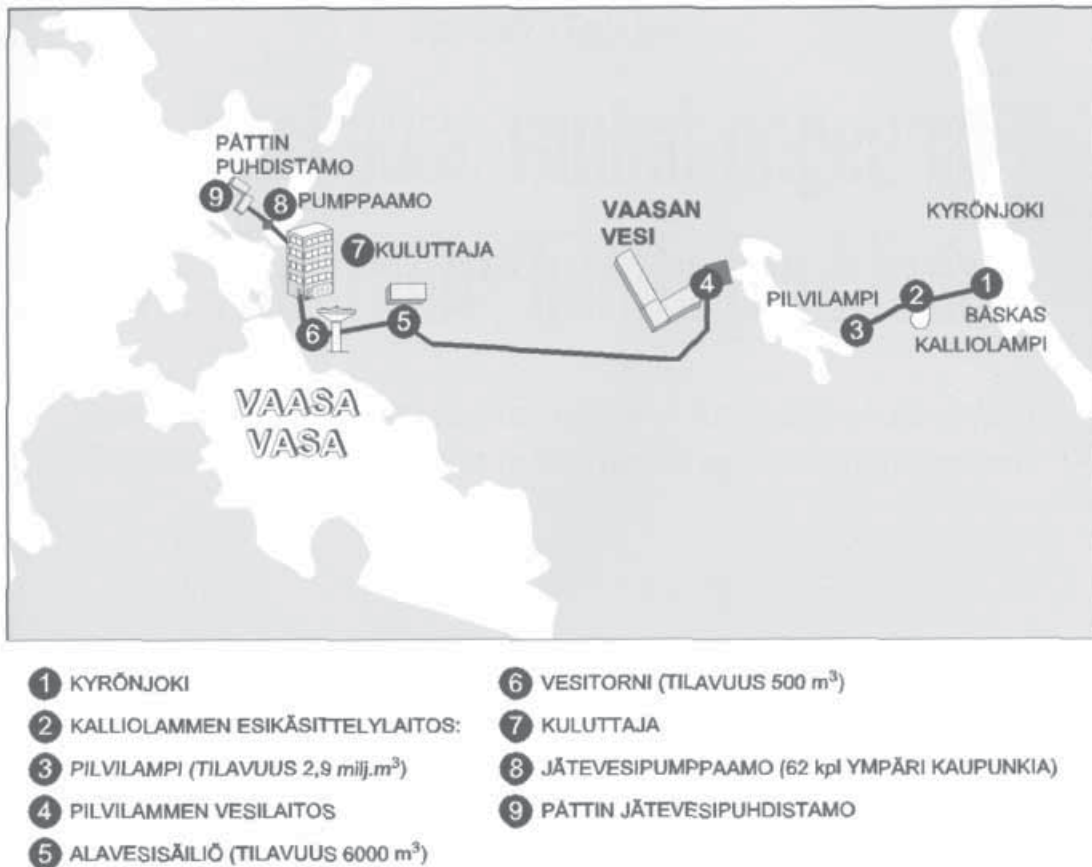
Figure 6. The overall cycle of water through the water supply and sewerage systems of Vaasa in 2005.
