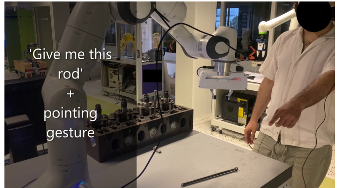
Fig. 1: Co-speech gesture model that combines a speech phrase, human gesture detection and object perception to command robot actions.
