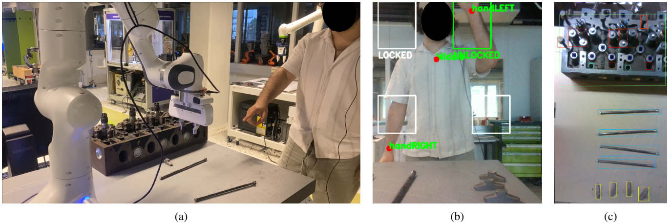
Fig. 3: Experimental setup with a human pointing at an object for robot picking (a). One camera is human front-facing to capture human hand gestures (b), one camera is mounted on the robot (eye-in-hand) for object detection on the table (c).
