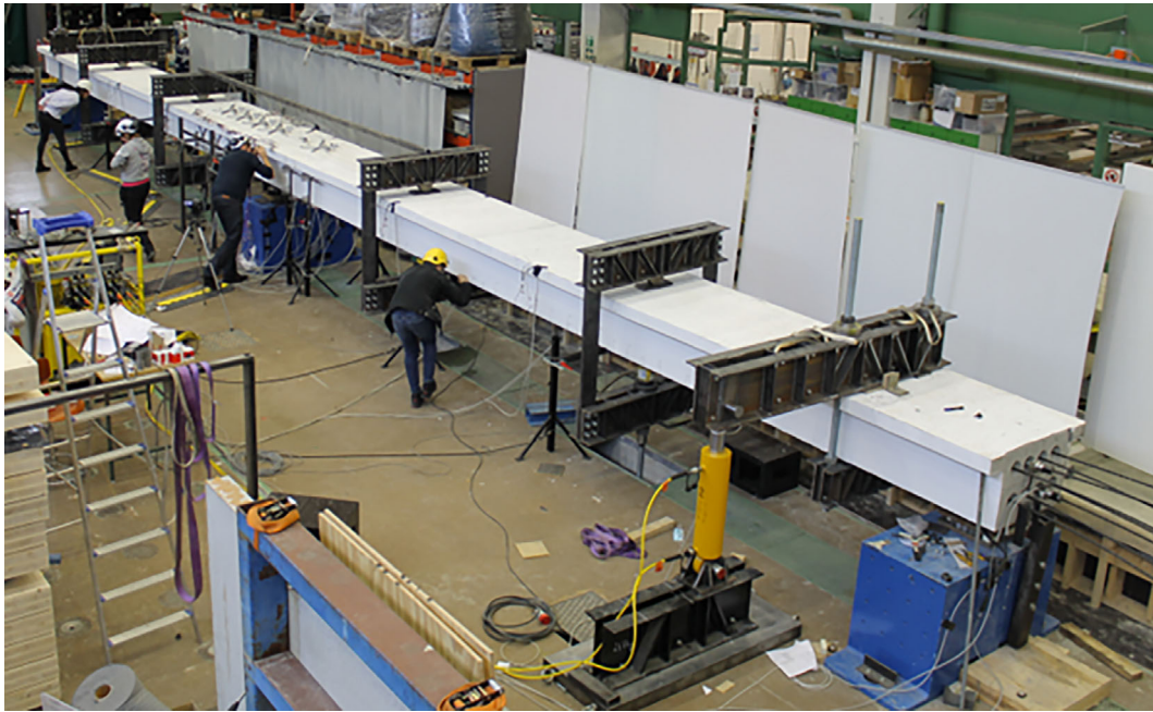
FIGURE 4 Test setup and instrumentation of test beam B4.
