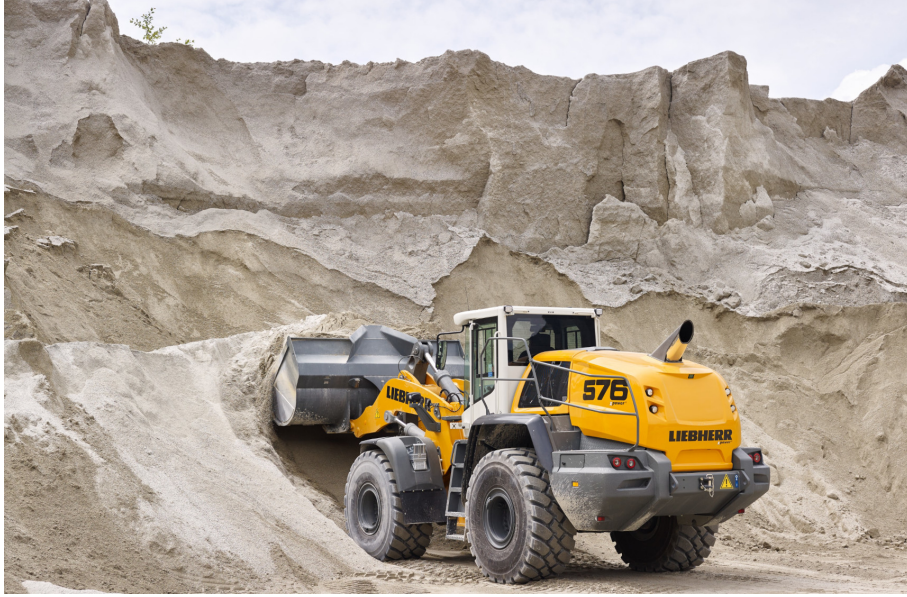
Figure 1: An L576 wheel loader loading sand [3].
