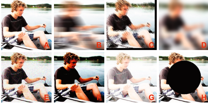
Figure 4.2 Distortions on the sample image. (A) Original image. (B) Motion blur. (C) Frosted glass blur. (D) Gaussian blur. (E) Noise. (F) Gamma darkening. (G) Gamma lightening. (H) Occlusion. Reproduced with permission from publication I (©2021 IEEE).
