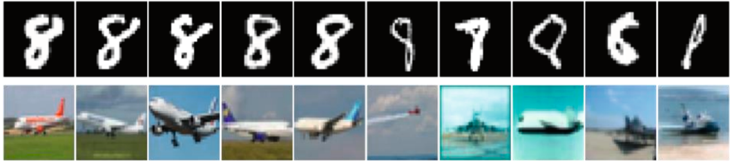
Figure 1: Samples of the same category in MNIST (Top) (Lecun et al. 1998) and CIFAR-10 (Bottom) (Krizhevsky 2009) datasets (Taken from (Chen et al. 2021)). From left to right, the difficulty of classifying is increasing for both manual and automatic label assignment, thus resulting in the increased chance of noisy labels.
