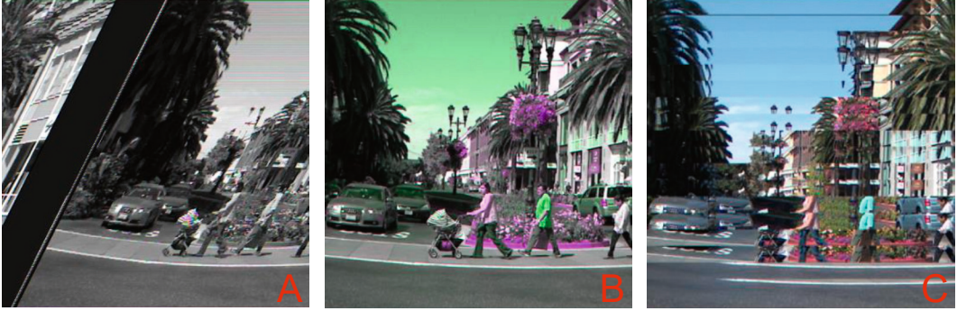
Figure 2: Effects of camera faults on the input image (Taken from (TND6233-D)): (A) Faulty clocking system, (B) Faulty pipeline, and (C) Faulty row addressing logic.
