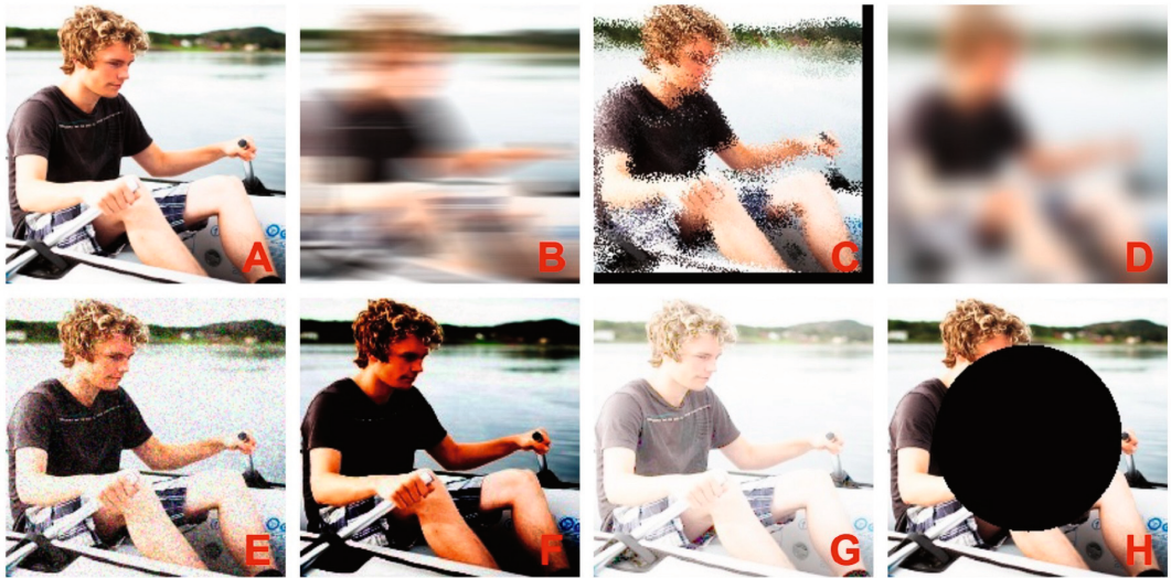
Figure 3: Effects of environmental factors on the input image (Taken from (Bakhshi Gerami, Rahtu, and Huttunen 2021)): (A) Original image, (B) Movement of camera/object (Motion blur), (C) Raindrop on the lens (Frosted-glass blur), (D) Out-of-focus object (Gaussian blur), (E) Low illumination (Gaussian noise), (F,G) Improper balance of light and darkness (Low/High brightness), and (H) Obscured object (Occlusion).
