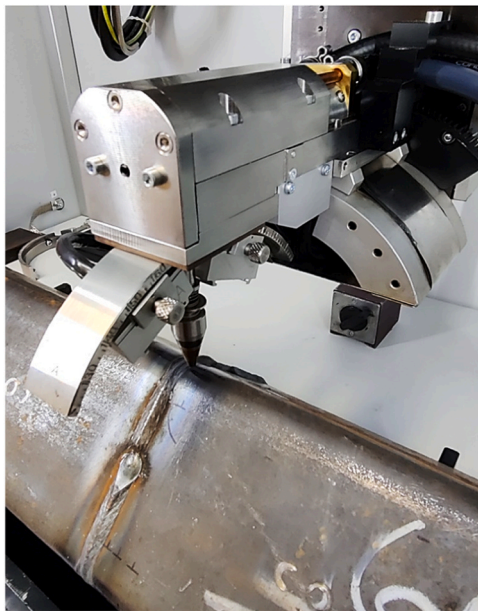
Fig. 3. Residual stress measurement of tube corner using Stresstech XStress 3000.
