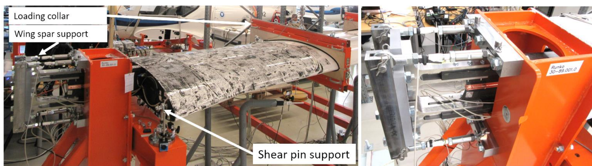
Figure 4: Wing support showing also the wing upper surface DIC pattern.
