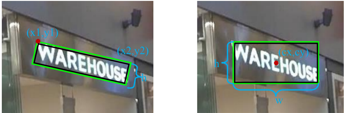
Figure 2.9. Oriented bounding box on the left. Horizontal bounding box on the right. From [26].
