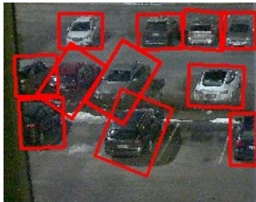
Figure 4.3. Actual ground-truth annotations, that are given to networks when training/evaluating
