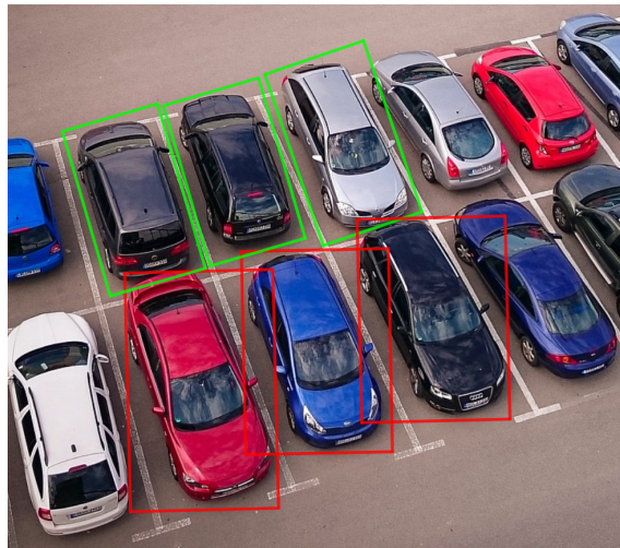
Figure 2.7. Oriented bounding box marked with green. Horizontal bounding boxes marked with red.
