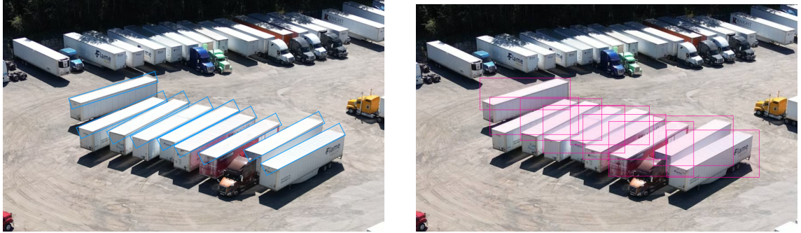
Figure 4.4. OBB annotations on the left are able to single out the trailers while the HBBs on the right can not.
