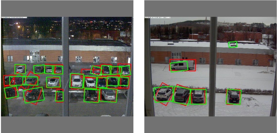
Figure 4.5. Ground-truth annotations in red and YOLOv5+CSL detections in green
