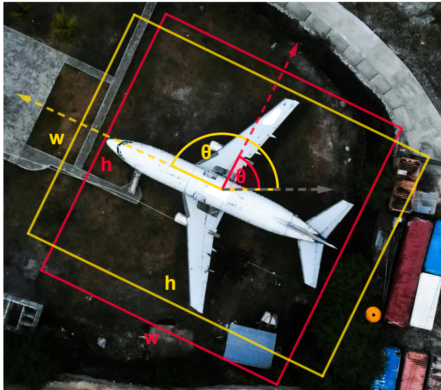
Figure 2.10. Boundary discontinuity problem of angle prediction. Red and yellow bounding boxes are similar, but they have very different angles, due to the fact that their longer and shorter edges are not on the same side. Adapted from [90].
