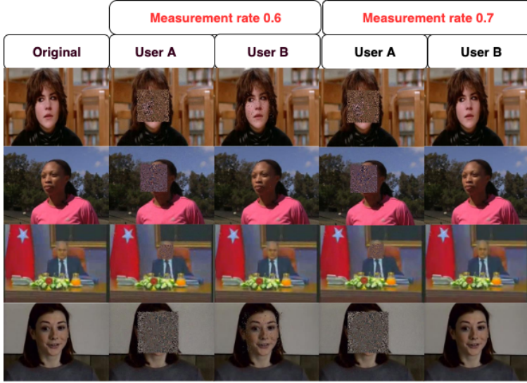
Figure 5.4 Example frames recovered for semi-authorized (User A) and fully authorized (User B) users at measurement rates of 0.6 and 0.7 [P4].
