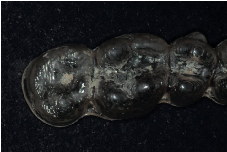
Figure 5. Images of retrieved aligner surfaces which are not completely smooth but exhibit microabrasions and irregularities(a). This may contribute to bacterial adhesion making the appliance more conducive to calculus accumulation(b).
