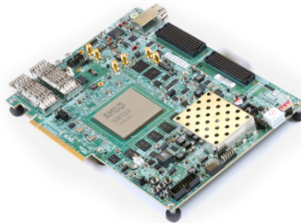
Figure 5.4. AMD-Xilinx VCU118 Development Board [2]
