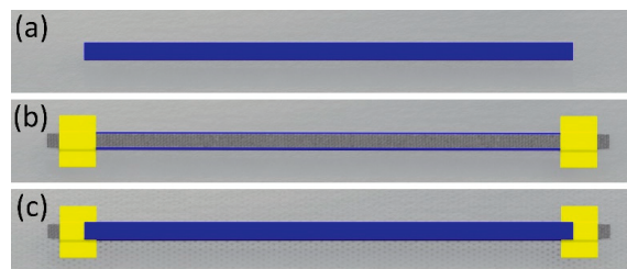
Figure 1. Preparation steps of the samples as modeled in Solidworks: (a) 3D printing of the sample's bottom half-layer, (b) placement of the CFC piece with the use of Kapton tape, and (c) continuing the 3D printing until the sample was ready.
