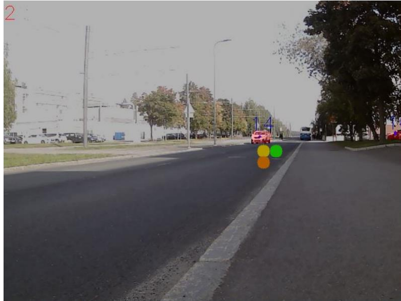
Figure 33 The Distant car is masked correctly but the radar data is not accurately calibrated to hit the car at a distance.
