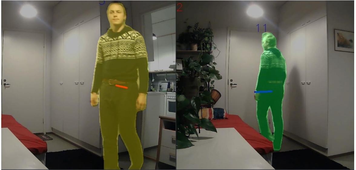
Figure 26 Demonstration of the true motion vector stemming from the true position of the calculated object center projected onto the image plane. To illustrate a 3D vector projection in the 2D image we encode motion towards the sensor with red and motion away from the sensor with blue.
