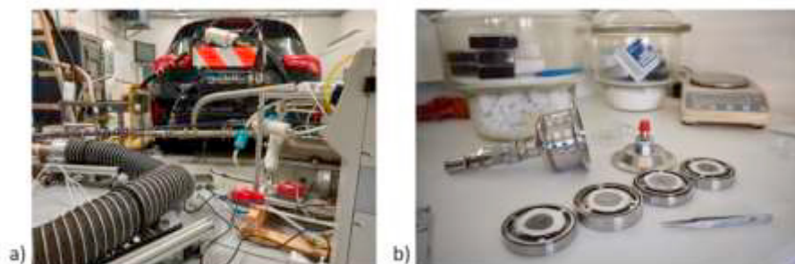
Fig. 5. (a) Installation of vehicle (gasoline direct injection vehicle equipped with a gasoline particulate filter) and measurement equipment at AUTH-Laboratory of Applied Thermodynamics. (b) Substrates of the DGI with collected particles.
