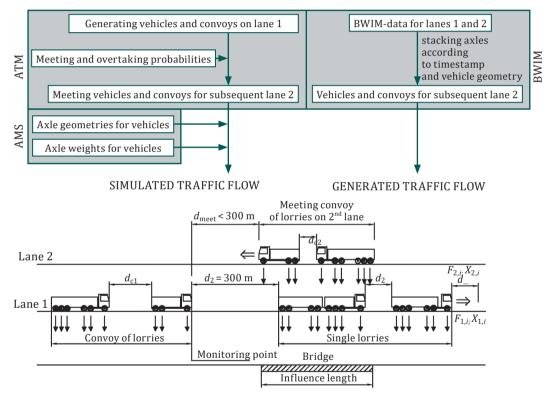
Note:  $d_{\text{meet}}$  - random distance of generated meeting vehicle on lane 2 (0 m <  $d_{\text{meet}}$  < 300 m);  $d_{c1,2,\dots,n}$  - intervehicle distance in convoy (5 m <  $d_{c1,2\dots,n}$  < 300 m), see Figure 3;  $d_2$  - intervehicle distance or distance between convoys (constant 300 m).
