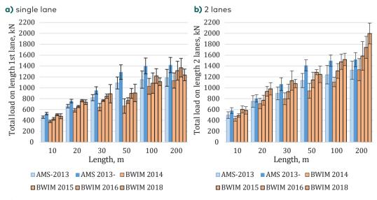
Figure 7. Simulation results vs. BWIM results of total load on influence length
