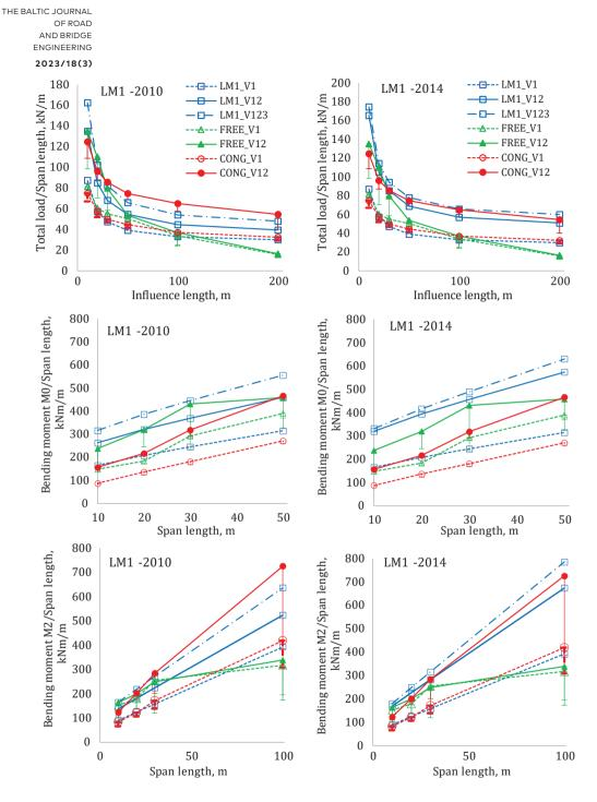
**Figure 11.** The selection of LM1 and calculated characteristic value of selected influence lines for free flowing traffic V1 and V12 and congested traffic V1 and V12
