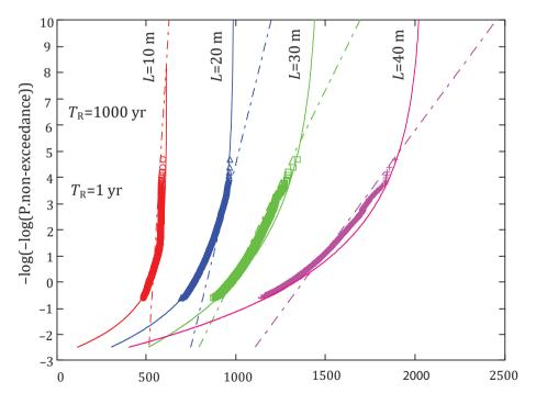
**Figure 10.** Simulated daily load effects and predicted extreme values for load effects for single lane V1
