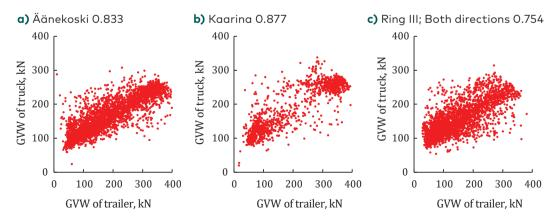
Figure 1. The correlation between truck and trailer for lorries with full trailer
