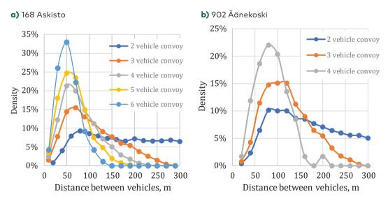
**Figure 3.** Distribution of intervehicle distance in convoys ( $d_{c1,2}$  in Figure 9) in ATM points
