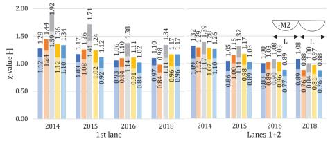
**Figure 9.**  $\chi$ -factors for a) total load on length; b) bending moment at midpoint; c) bending moment on middle support of 2-span beam for 1<sup>st</sup> lane and combined effect of lanes 1+2, in Äänekoski
