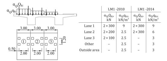
Figure 12. The selection of Load Model LM1
