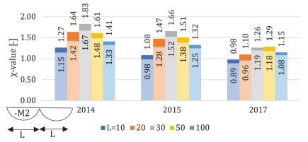
**Figure 8.**  $\chi$ -factors for total load on length, bending moment at midpoint of single span, bending moment on middle support of 2-span beam in Askisto
