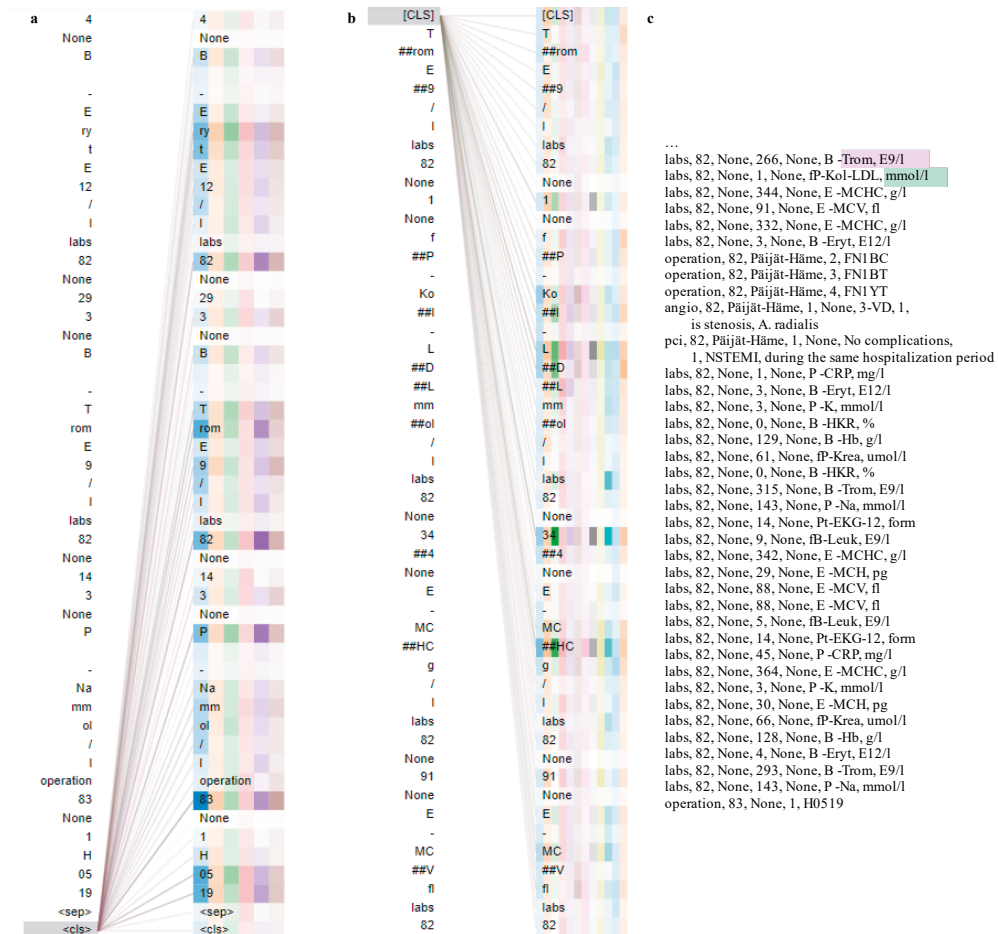
Figure 5.5 The attention weights in (a) XLNet and (b) BERT in selected layers (5th and 12th respectively) near the CLS token, for a given example of a positive case, correctly classified by XLNet and misclassified by BERT. The example is shown in text form in (c) with the first information available for XLNet and BERT highlighted in green and purple, respectively.
