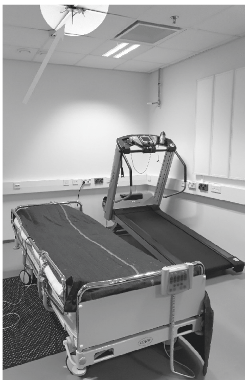
Figure 3. The measurement setting. The FMCW radar (highlighted in brighter tones and pointed out with a red arrow) is mounted on the ceiling above the bed. The treadmill beside the bed was used for exercising during the measurement session.
