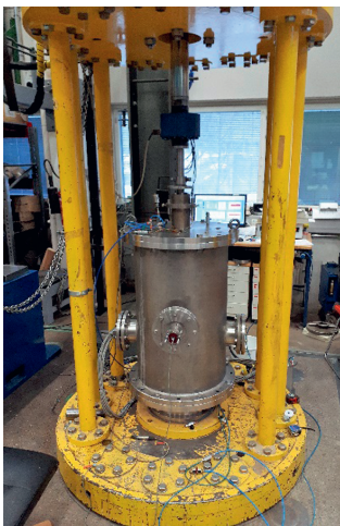
Fig. 3.2. Large-scale test equipment used in the cyclic load triaxial test. Specimen dimensions were d = 200 mm and h = 400 mm.
