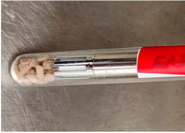
Figure 2. Test tube with LDF material in small pieces and humidity probe.
