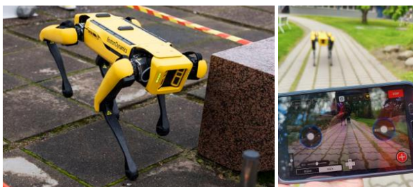
Figure 1. The Spot robot and its operating mobile application used in the outdoor physical activities of the field study.
