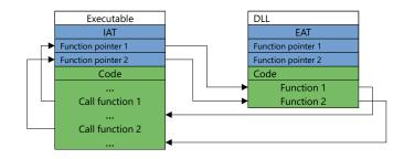
Figure 3.2. Program flow without IAT hooking, adapted from figure in [22].
