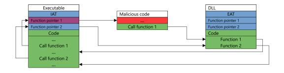
Figure 3.3. Program flow with IAT hook in place, adapted from figures in [22] and [7].
