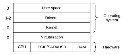
Figure 3.1. Simplified operating system architecture
