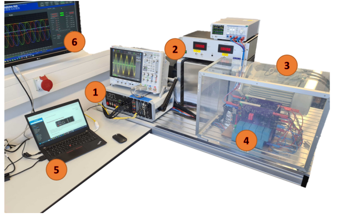
Fig. 6: Lab testbench: 1: UltraZohm , 2: Load machine, 3: Six-Phase PMSM, 4: Two-level SiC-inverters, 5: Host computer, 6: Graphical user interface
