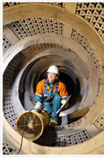
a Image description: Field service employee checking trommel screen inside the mill at a mine in Canada. Copyright: Metso Corporation
