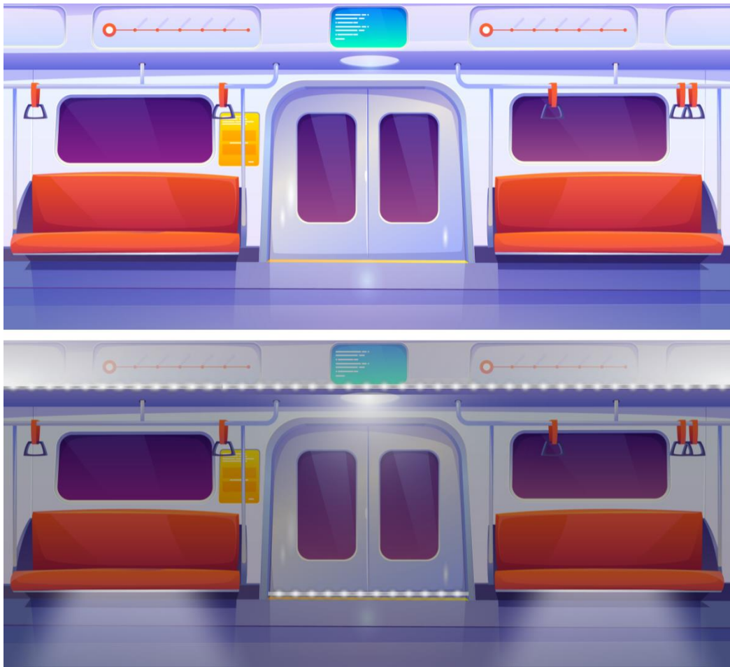
Figure 8. Two different lighting situations. Above, bright lights reflected from the surfaces of the vehicle. Below, dimmer lighting, with lights placed under the benches to help people move around, lights on the hat racks pointing to information boards. Above the door and on the threshold, lights to facilitate safe passage. A sense of security must be ensured by decreased lighting and routes must be clearly marked and illuminated.
