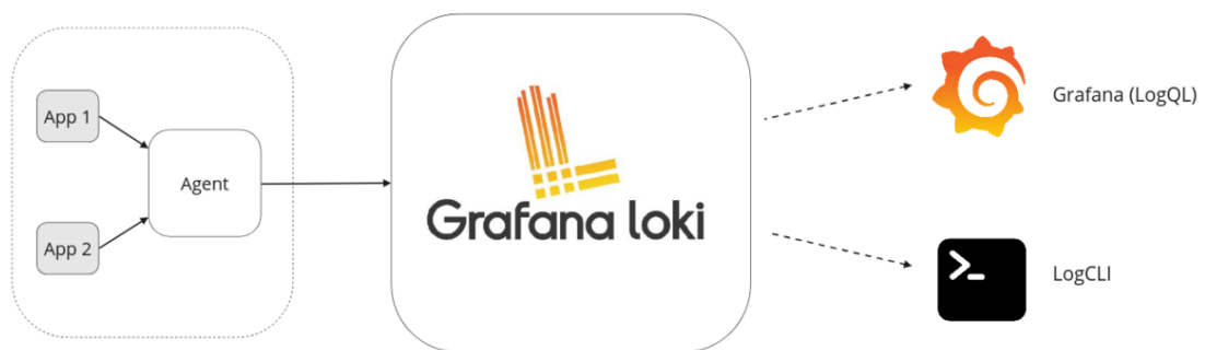
Figure 4.3. The architecture of Grafana Loki
