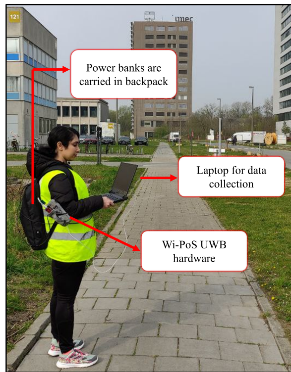
Fig. 1. The pedestrian carrying the setup in an open outdoor environment. She walks on a predefined route for 10 minutes with speed of 6\text{km/h} in each environment.
