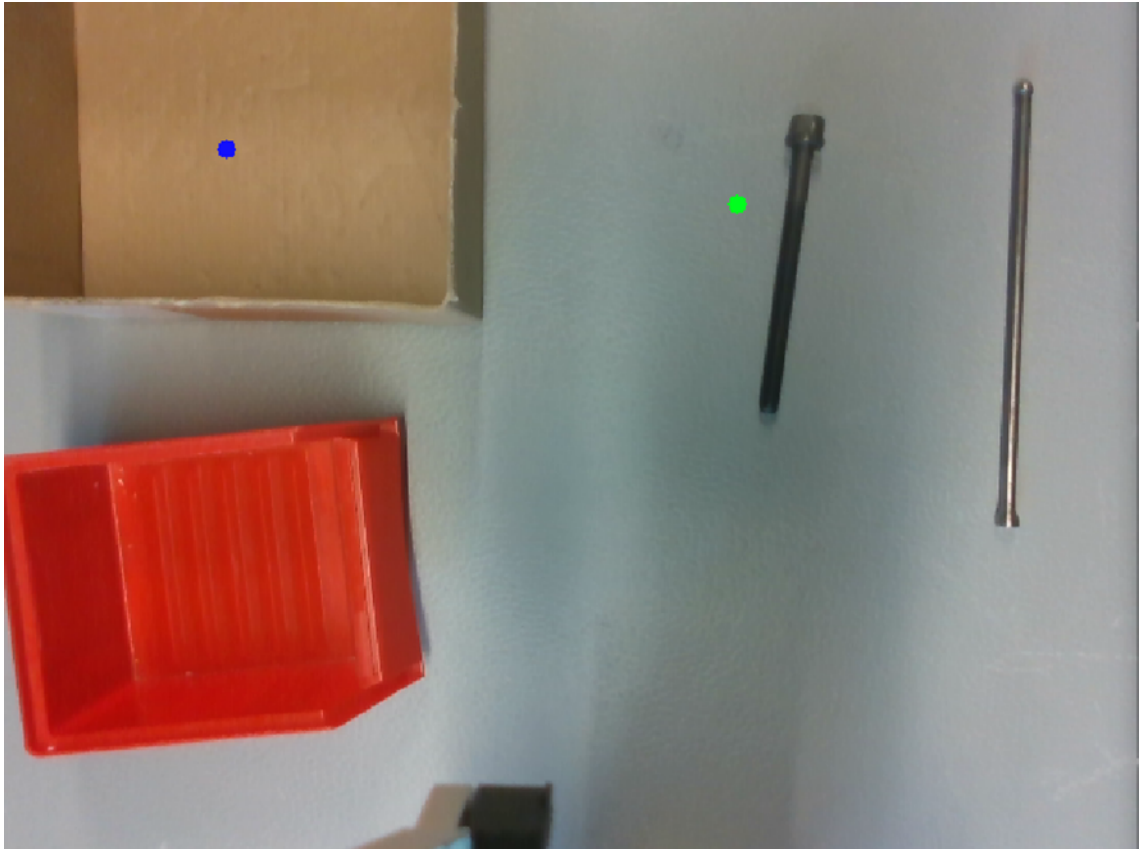
Figure 4.4. RGB image view for “put bolt in brown box” with pick position (green dot) and place position (blue dot) from the left lens of the D435 camera.
