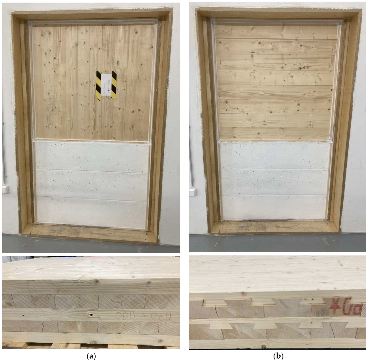
Figure 5. Mounting of test specimens: (a) CLT; (b) DMWBE (photos by authors).
