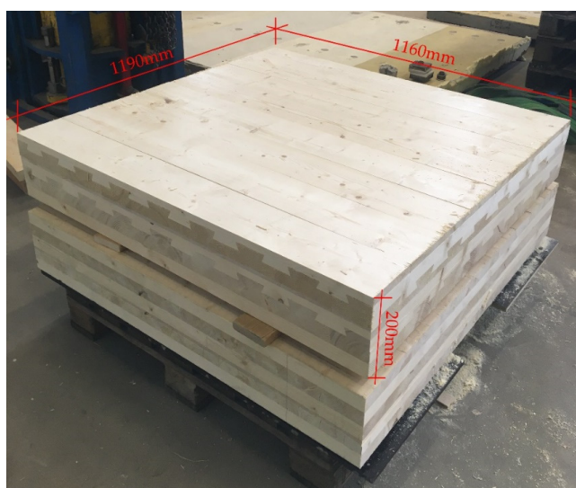
Figure 2. Test specimens: DMWBE ( upper ) and CLT ( lower ) (photo by authors).
