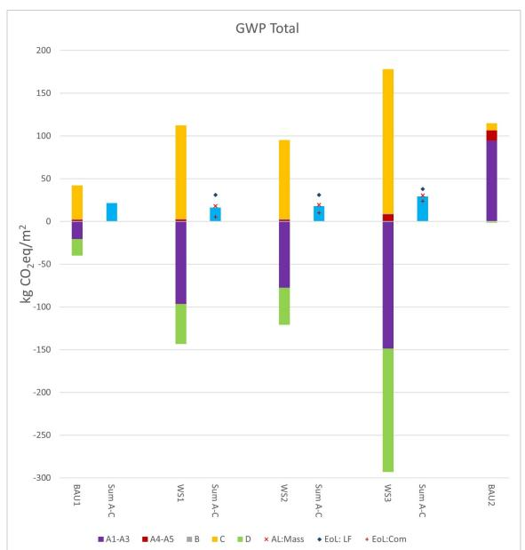
**Figure 7.** Total GWP of studied wall structures. In the base case, the allocation method in WS is cut-off, and the drying energy source in WS + C is grid mix. Thick marks show the sum of GWP when using the alternative allocation method in WS (AL: mass = impact allocated according to masses) and the sum of GWP when using the alternative EoL scenarios in WS (EoL: LF = landfilling as an EoL scenario, EoL: Com = composting).
