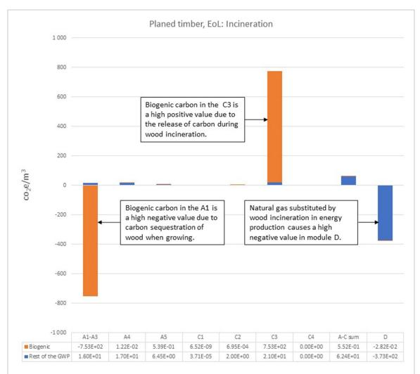
**Figure 2.** The logic of biogenic carbon and module D in EN 15804 is explained by illustrating data from EPD of planed timber by Stora Enso with incineration as an EoL scenario (EPD International 2020a). The negative value in A1–A3 illustrates the carbon sequestration of wood when growing, and the high positive value in C3 illustrates the release of carbon storage when incinerating the wood in the EoL phase. A–C sum sums up the impact of the product system under study.
