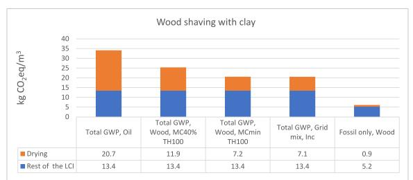
**Figure 4.** Impact of drying energy options to GWP of WS with clay. EoL scenario in all the cases is incineration. MC refers to the moisture content of wood chips in storage. TH100 refers to the TH used in assessing the biogenic carbon cycle in wood chip incineration. 'Rest of the LCI' refers to the life cycle GWP excluding the impact of drying energy.
