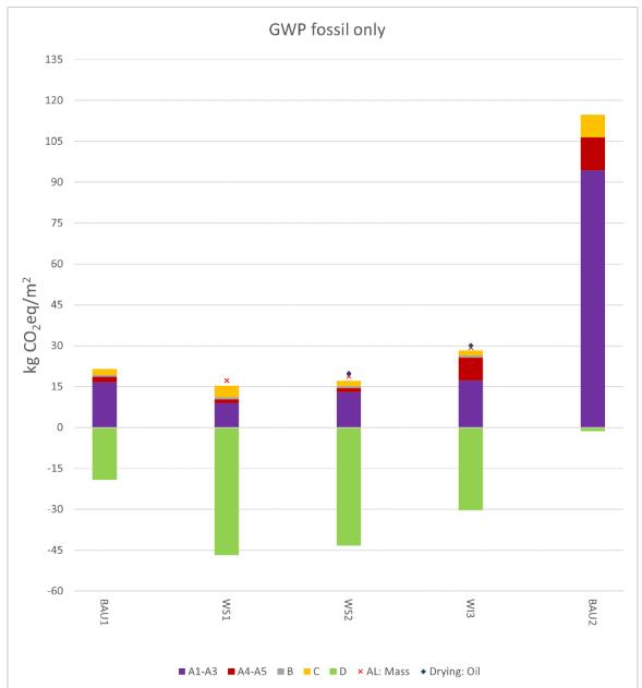
Figure 6. Fossil GWP of studied wall structures. In the base case, the allocation method in WS is cut-off, and the drying energy source in WS + C is wood chips. Thick marks show the sum of GWP when using the alternative allocation method in WS (AL: mass = impact allocated between main product and WS according to masses) and the sum of GWP when using the worst scenario in drying energy of WS + C (Drying: oil = heating oil as an energy source in drying).
