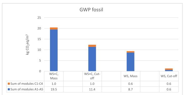
**Figure 3.** Impact of the allocation approach to the fossil GWP of insulation made of WS and WS with clay. The drying energy of the WS with clay is the grid mix. The EoL scenario in all the options is incineration. 'Cut-off' refers to the case where the study applies the cut-off approach when calculating the product phase impact of WS, and 'Mass' refers to the case in which the study allocates the burden between WS and timber according to masses.
