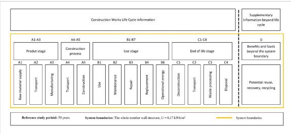
Figure 1. System boundaries of the study and life cycle phases in the building's LCA according to EN 15804.
