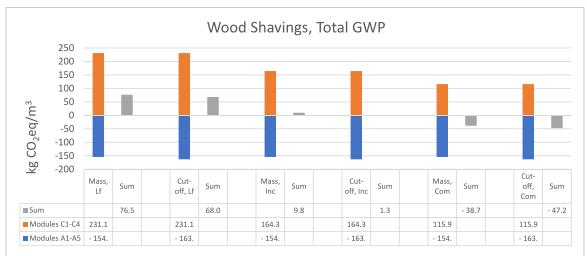
**Figure 5.** Impact of EoL scenario and allocation approaches to total GWP. EoL scenarios: landfill (LF), incineration (Inc), composting (Com). Allocation approaches: cut-off allocates all the product phase impact to planed timber, and mass allocates the impact between WS and planed timber according to the ratio of output mass. In the table, A refers to product phase impacts, and C refers to EoL phase impacts. 'Sum' refers to the whole life cycle GWP of the material under study.
